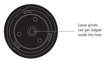
To dislodge loose grinds, remove each of the removable grind containers in turn and shake the main power unit to release any loose grinds. There is no need to empty the containers. Replace the grind containers and use as normal.
